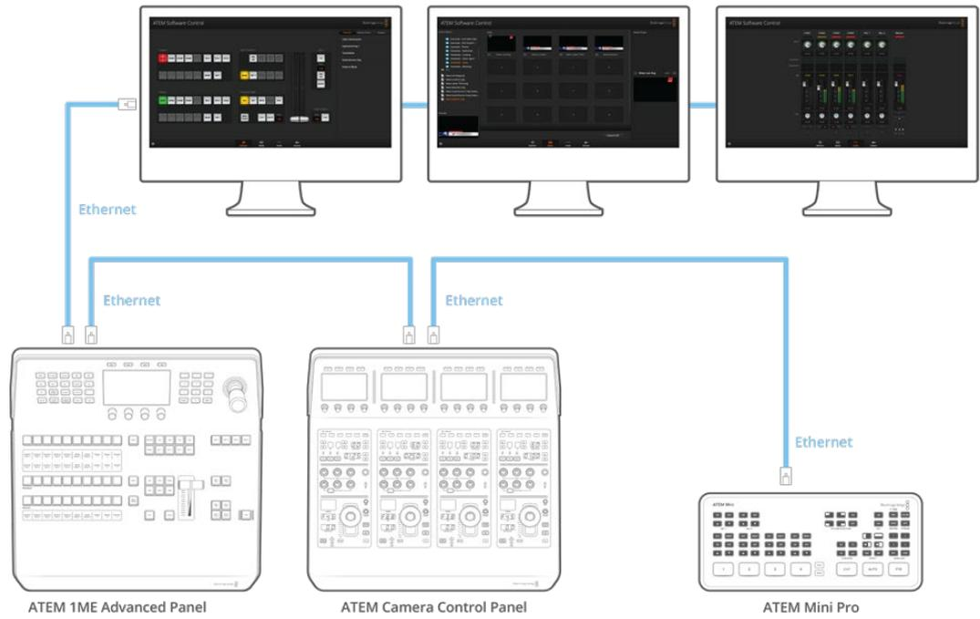
When connected to a network via Ethernet, multiple computers can run ATEM Software Control simultaneously, which means multiple operators can be dedicated to separate controls on your ATEM Mini. For example, multiple operators can control media management, camera control and audio mixing.
