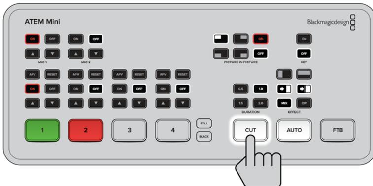
In program preview switching mode, press an input button and then press the 'auto' or 'cut' button to switch the source to air
