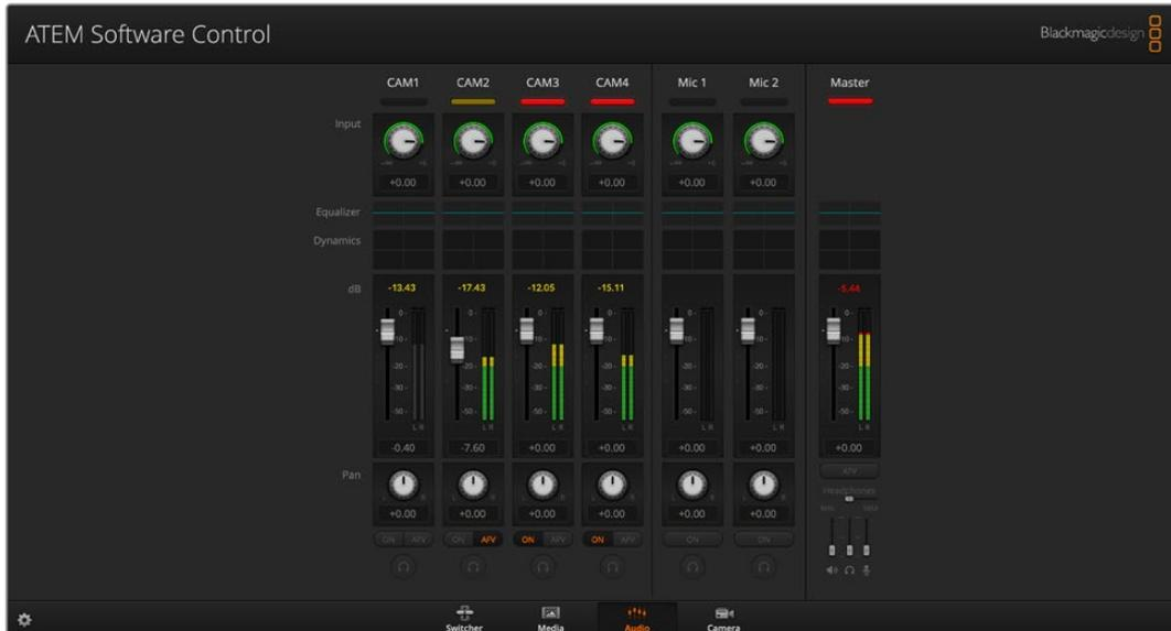
Your ATEM Mini also features built in mic inputs for mixing external audio.
