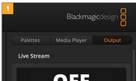
In ATEM Software Control's processing palettes, click on the 'output' tab. Open the 'live stream' palette.
