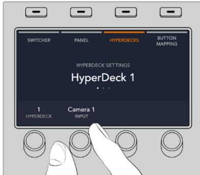
Repeat this process for any additional HyperDecks you have connected to your switcher by assigning inputs to HyperDeck slots 1, 2, 3 and 4, if required.
