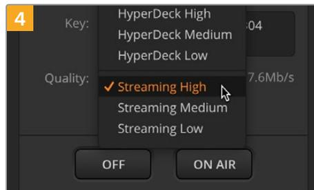
Set the streaming quality to low, medium, or high. This will also set the quality for the recording output via USB-C.
