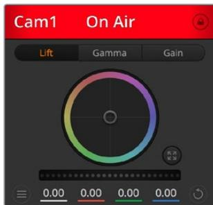
Each camera controller displays the channel status so you know which camera is on air. Use the color wheels to adjust each YRGB channel's lift, gamma and gain settings.
