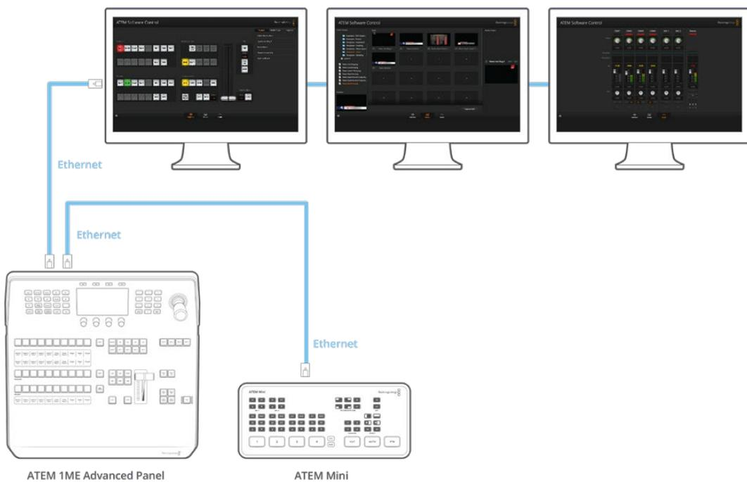
Multiple computers can run ATEM Software Control simultaneously, which means multiple operators can be dedicated to separate controls on your switcher, for example media management and audio mixing.
