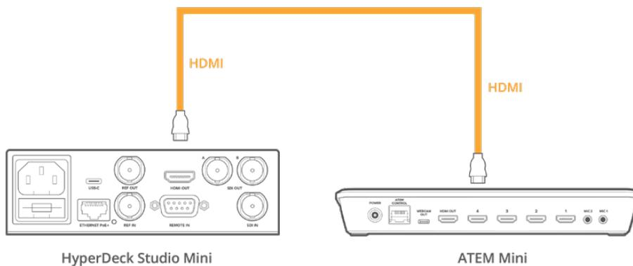
Plug the HDMI output of a HyperDeck Studio Mini into one of your ATEM Mini's HDMI inputs
