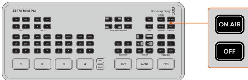
The stream buttons labelled 'on air' and 'off' let you start and stop streaming directly from your ATEM Mini Pro
