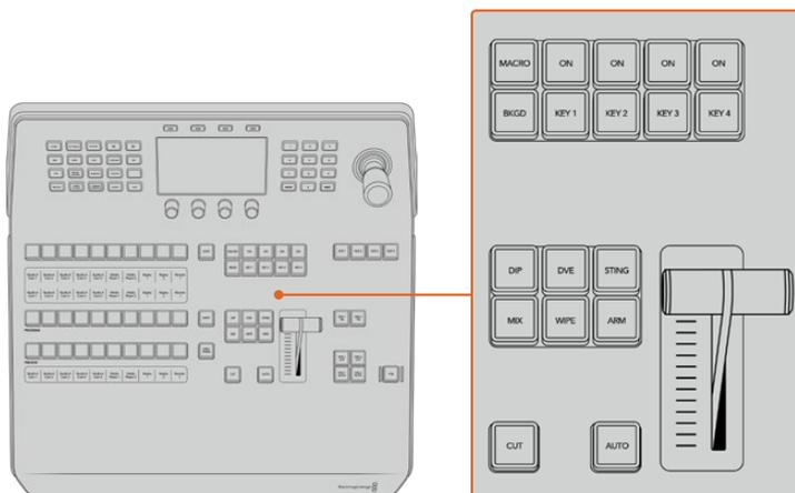
Press the button marked CUT in the transition control block to perform a cut transition
