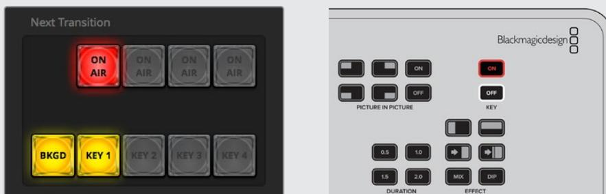
Changing the 'on air' setting in the LCD menu also changes the state of the 'on air' next transition button in ATEM Software Control
