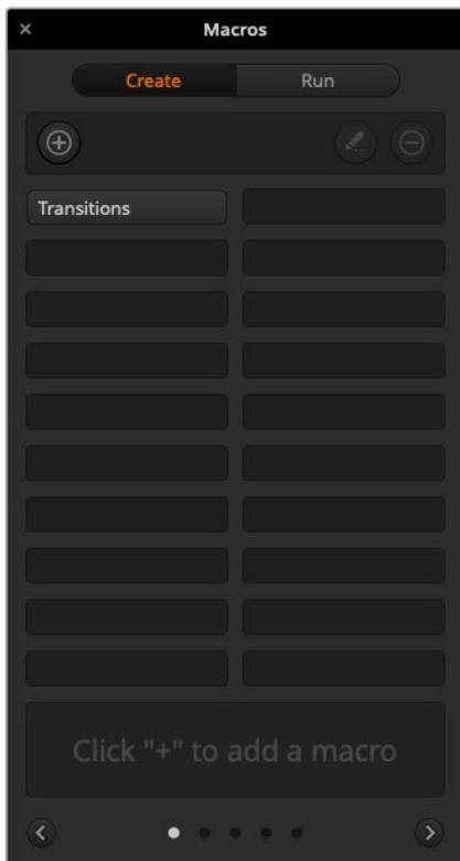
The image shows how a macro button appears in the macros window after it has been recorded. To run a macro, click on the 'run' button to enter the run page. Now you can load and/or run the macro by clicking on the macro button.
