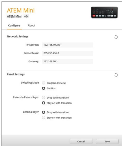
Change network settings using the 'configure' tab in Blackmagic ATEM Setup.
