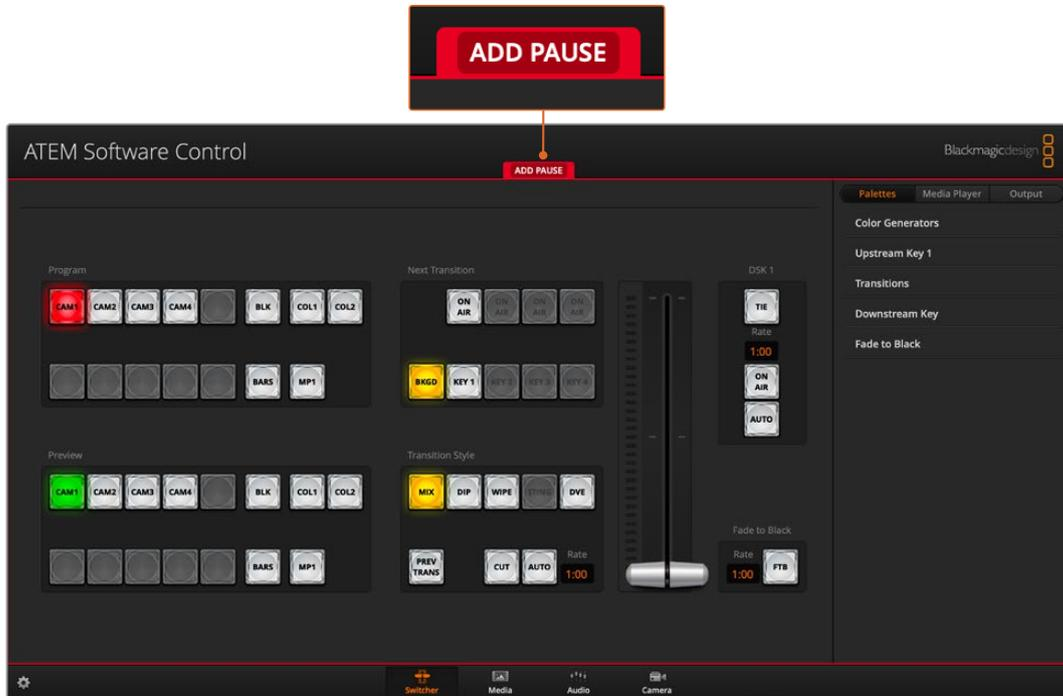
ATEM Software Control displays a red border to indicate when you are recording a macro. The 'add pause' button located at the top of the red border lets you enter durations for pauses between switcher actions.
