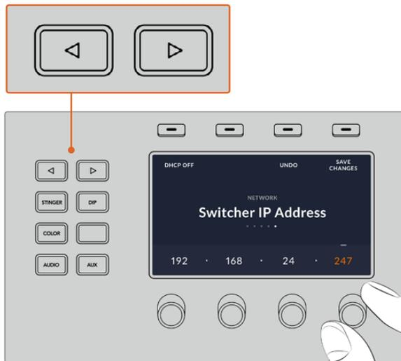
On the ATEM 1 M/E Advanced Panel, press the 'network' LCD soft button to open the network settings on the LCD, then use the system control arrow buttons to navigate to the switcher IP address setting. Use the soft controls to set the network IP address for your switcher, and don't forget to save the changes.
