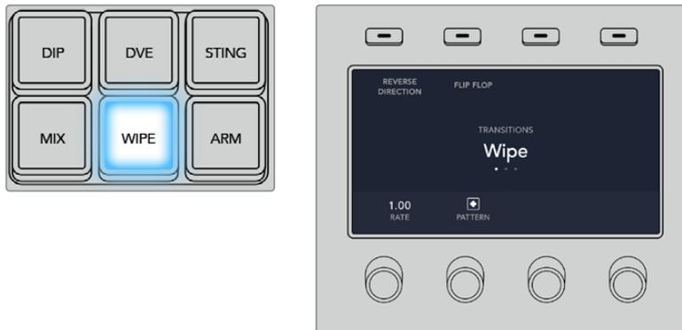
Press a source button in the source select row to select a source for the wipe border. Hold the shift button down to select a shifted source, such as a color generator or media player.
