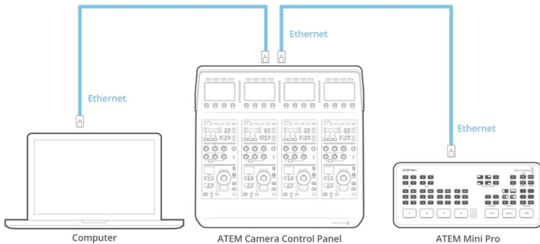
After connecting the camera control panel to your ATEM equipment, you should see the lights on the panel illuminate and the LCDs on each CCU will display their respectively assigned cameras. The panel is now powered, connected to your switcher and ready to start controlling your cameras!
