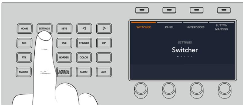
You'll notice that ATEM 1 M/E Advanced Panel displays four setup options along to top of the LCD screen. These include 'switcher,' 'panel,' 'HyperDecks,' and 'button mapping.' Each corresponds to a setup menu. Simply press the LCD soft button above 'HyperDecks' to enter the 'HyperDeck settings' menu.
