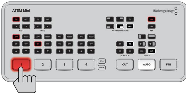
In cut bus mode, pressing an input button will instantly switch it to air
