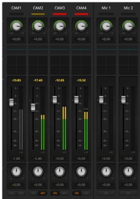
Try sliding the gain faders up and down on your hardware control surface and verify that the audio mixer faders show a corresponding movement in the software on your computer screen
