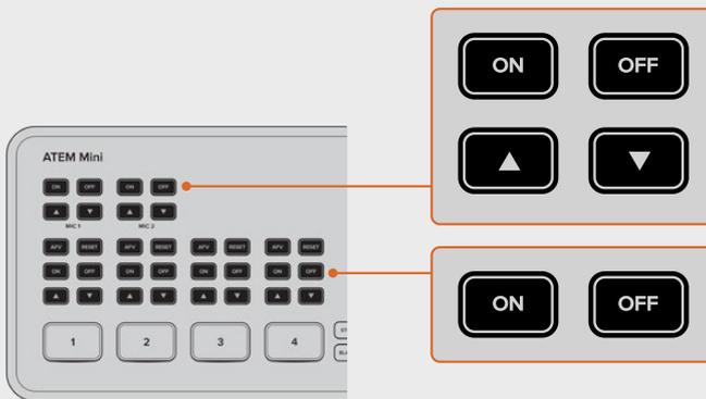
**ON** – When the input's audio is set to 'on', the input audio will be heard permanently, even if the source is not currently on air.
