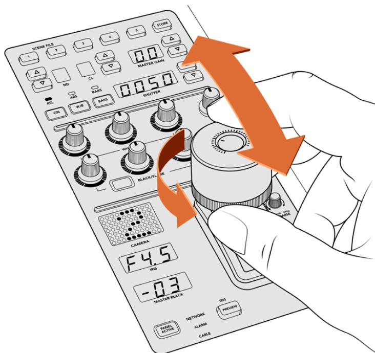
The joystick lets you adjust the gain level by leaning the controller forwards and backwards. The master black level can be adjusted by turning the ring wheel clockwise or counter clockwise. Corresponding indicators are provided for accurate measurement.
