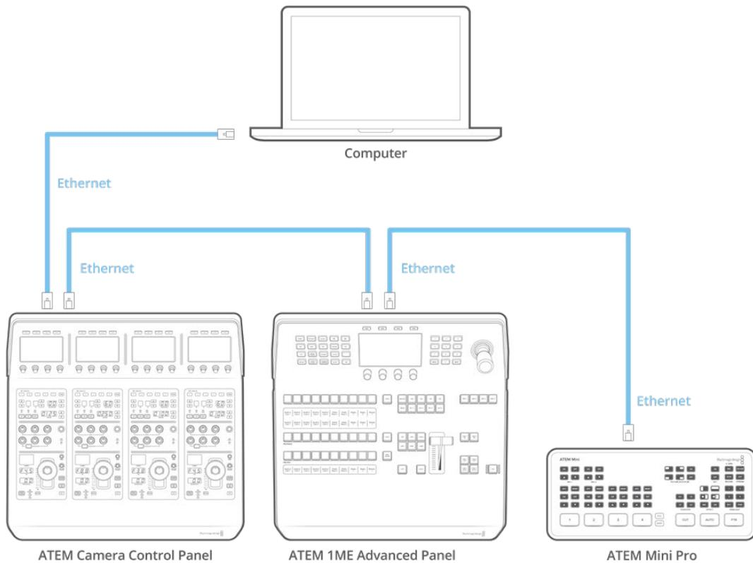
If you are using the camera control panel with just your switcher and a computer on a shared network, connect the panel to your switcher, then the spare Ethernet port to your computer.
