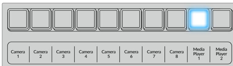
Press a source button in the source select row to select a source for the wipe border, such as a camera or media player.
