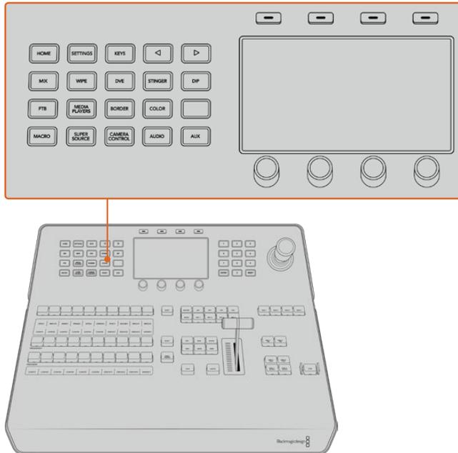
Change network settings using the system control buttons and LCD soft controls
