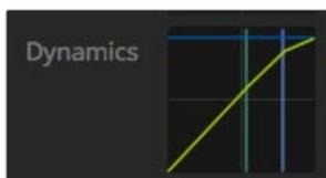
The dynamics controls can be opened for each input and the master output by clicking on its corresponding dynamics indicator
