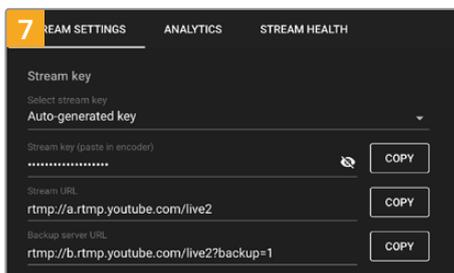
An auto generated stream key will appear in the stream settings, click 'copy' to copy the stream key.
