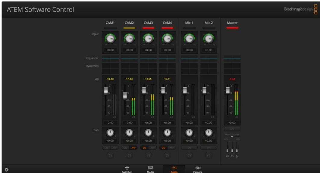
This section of the manual shows the different Fairlight audio controls you can use to shape and optimize the audio mix in your live production.
