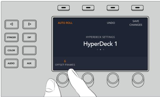
As HyperDecks must buffer a couple of frames before commencing playback, the actual cut will be delayed a preset number of frames to ensure a clean transition. This is just like setting a preroll on a videotape machine. You can adjust the length of this delay by changing the 'offset' frames number using the control knob under this indicator. Press the soft button above the 'save changes' indicator to confirm your change.
