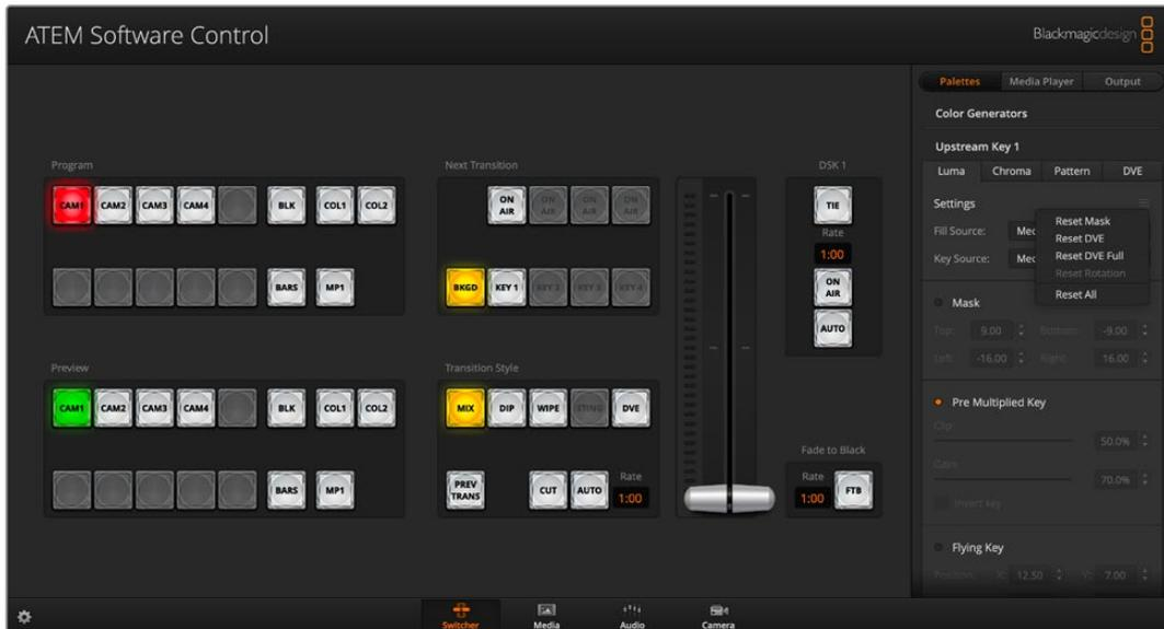
ATEM Software Control is included in the ATEM software installer and can be downloaded from the Blackmagic Design website. It's free and allows you to control your switcher in a similar way to a full hardware control panel. A range of palettes on the right side shows you all processing features of your ATEM Mini and allows settings to be easily made.
