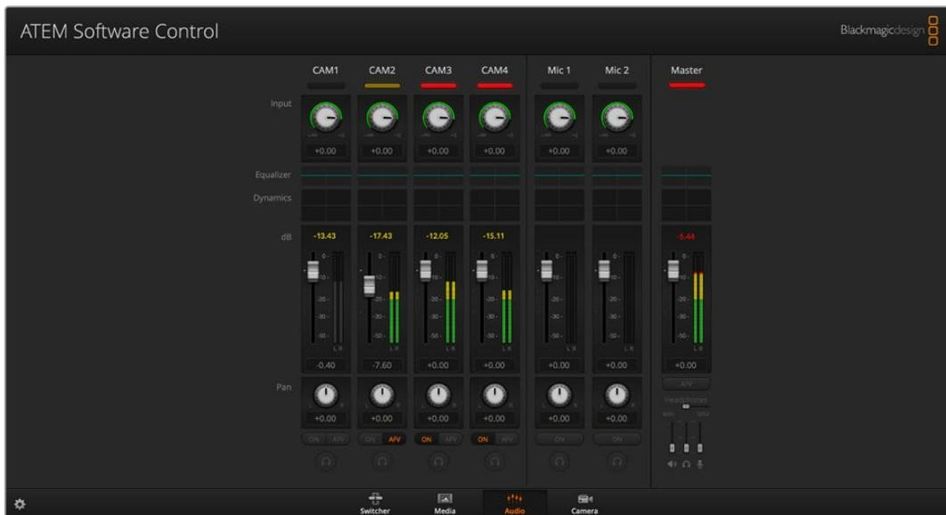
The audio mixer displays tally lights for any audio sources that are currently on air or when AFV is selected, as well as audio level, audio balance and buttons for selecting which audio should be used
