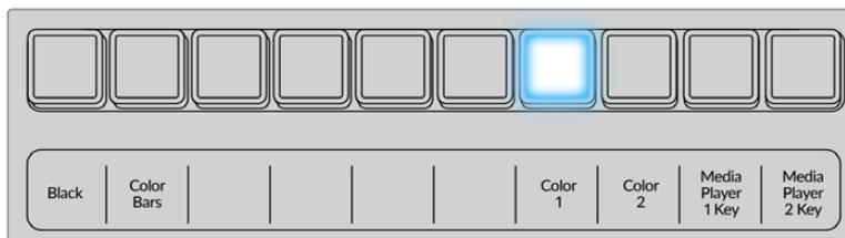
Hold the shift button down to select a shifted source, such as color bars or a color generator.
