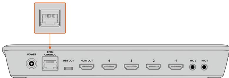
Connect ATEM Mini to a network and then you can operate your switcher using ATEM Software Control on any computer connected to the same network
