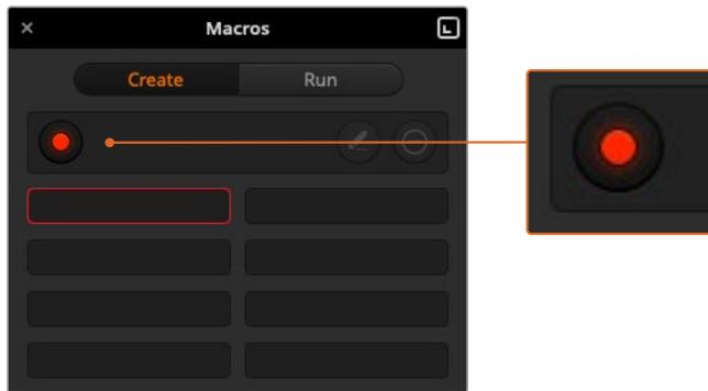
While recording, the create macro button will change to a 'record' button. When you have completed your switcher actions, click on the 'record' button to stop recording.
