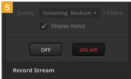
With all the streaming details now set, it's worth performing a quick test broadcast to make sure everything is working. Press the 'on air' button on ATEM Mini Pro, or click on the on air button in the live stream palette.
