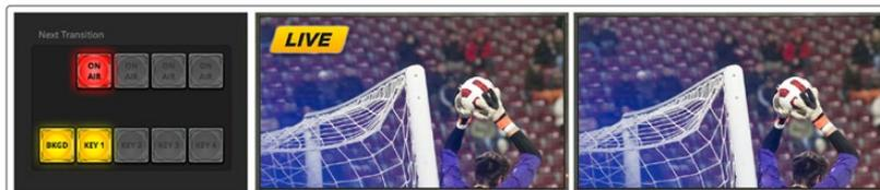
There are multiple ways to transition a key to the program output. The key can be cut on or off, it can be mixed on or off, or it can be mixed along with a background transition. Upstream keys are transitioned to the program output using the next transition controls. Downstream keyers can be transitioned using their own transition buttons or by using the DSK TIE buttons to link the transition with the main transition.
