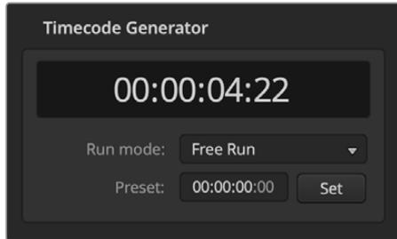
When using ATEM Mini Pro, the timecode generator can be set to time of day, or free run timecode where you can set a manual preset timecode
