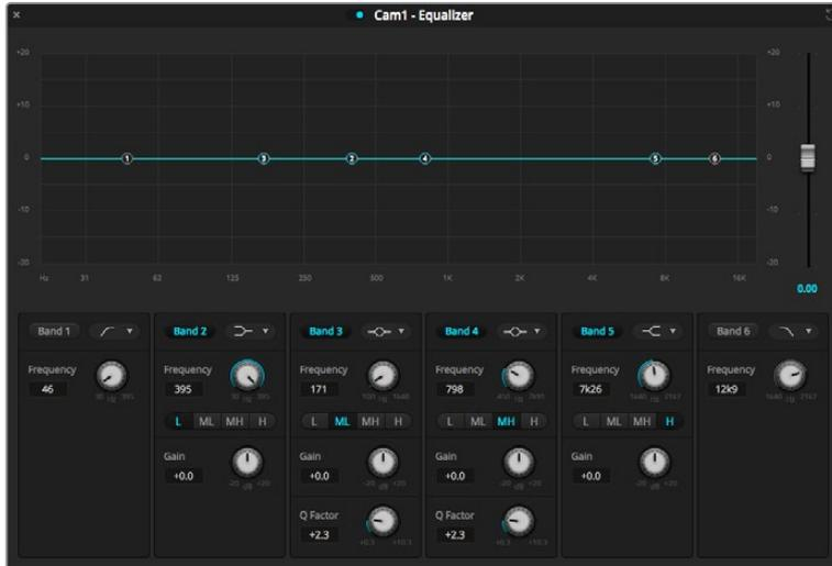
Each audio input has its own 6 band parametric equalizer
