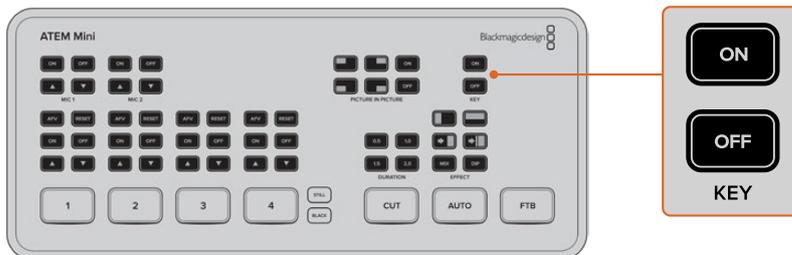
Press the 'key' on or off buttons to switch the upstream keyer on and off air
