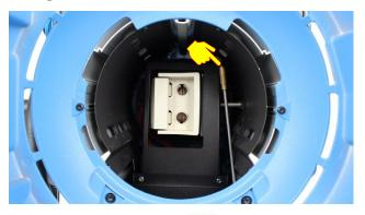
After removing the lens door, and the reflector, you must pull the SSA backwards into the housing and leave in the position as shown. Please follow the instructions in the safety switch activator section.
