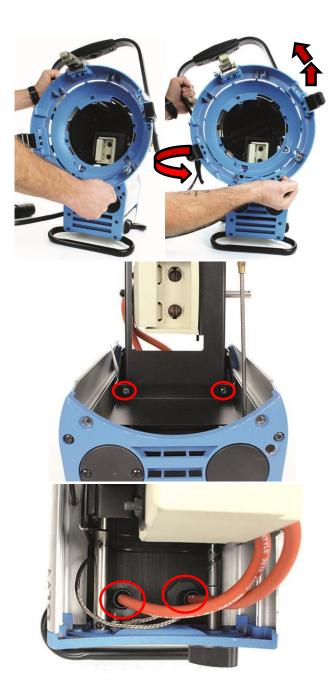
Place one hand on the skid and pull the housing upwards from the stirrup (it can hang on the lamp lock shaft, you may need to wiggle the housing). Lean the housing to the left to remove completely.
