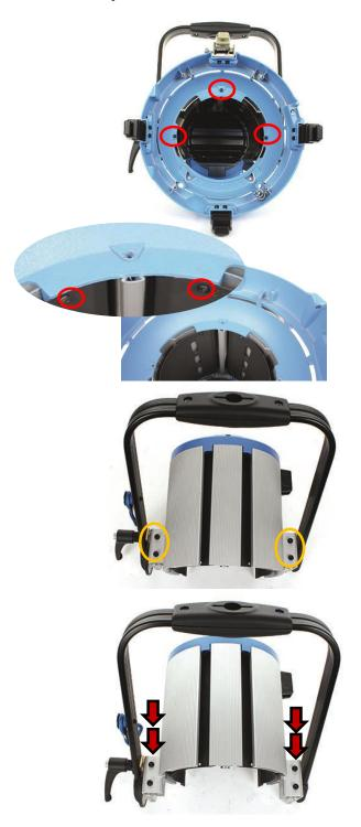
Remove lens door, reflector, SSA and housing Remove 3 screws on the inside of the front casting (Torx 20.)
