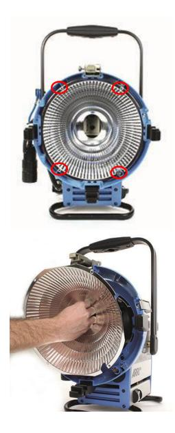
Remove 4 screws (Torx 20) around the reflector rim.
