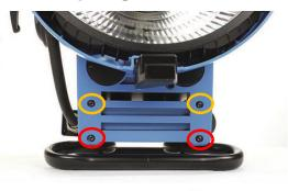
Remove the 2 screws on the bottom/front (marked in red.) Loosen the 2 middle screws (marked in yellow.) Do not remove.
