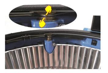
Make sure there is enough space between the SSA (brass) and SSA pin plate (silver) Please refer to the picture. Listen for a 'click' sound. It should click twice before the door latch closes. If this is not adjusted properly than the safety loop can be opened and the lamphead will not strike.
