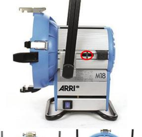
Remove the screw (Torx 20) of the lamp lock knob. Loosen the screw and remove completely.
