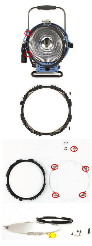
Loosen and remove two screws (Torx 10) to remove the lens door from the housing.
