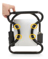
Tip: To reassemble loosen all 4 screws of the skid. This alows a better fit for the base group and the housing.
